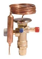
a new family of valves RFGD, that can be considered a natural evolution of the range RFGB. RFGD valves have fixed orifices, a straight layout, solder ODF connections and are available for 5 refrigerants types included R410A. With a capacity range from 12.3 kW to 45kW (conditions: *R410A*, *Condensing temperature: 38°C; evaporating temperature +4,4°C; Liquid temperature 37°C Static Super Heating: 3,5K*).
